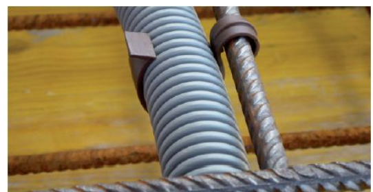
The tube is pushed into the big opening, with the small opening attached to the wire. Fixings in the small opening prevent the clip from sliding.
